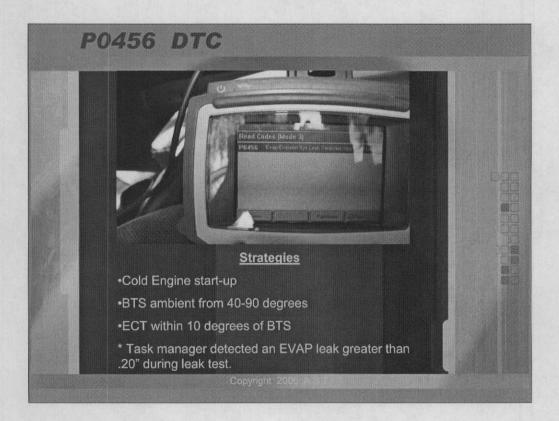
The stored DTC was a P0456, which upon looking in my Mode \$06 diagnostics manual, I was able to determine that the code referred to a small leak present in the EVAP system. I also learned the code setting criteria needed to set this DTC. This may become useful information to aid in getting the monitor to run after the repair has been completed.
