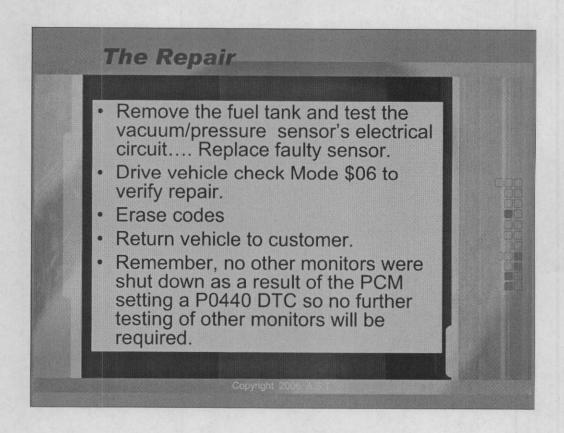
At this point I decided I needed to remove the tank and perform some circuit and component testing on the fuel tank pressure sensor itself. I was able to determine that the circuit was fine and that the sensor itself had failed. Replacing the sensor had successfully repaired this vehicle.
