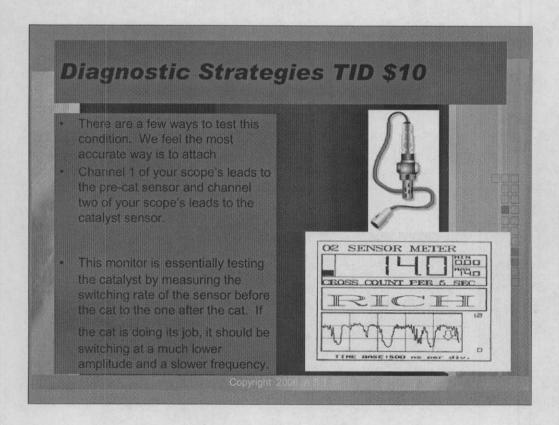
There are a few ways to test this condition. We feel the most accurate way is to attach
