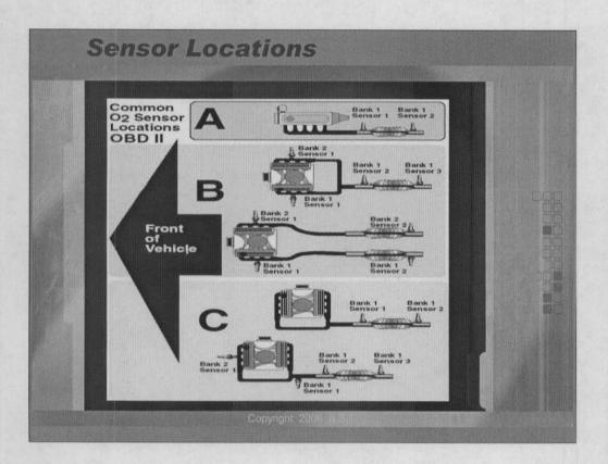
We should start by identifying the oxygen sensor locations. We have supplied you with a graphic showing the various locations of each of the sensors located on various engine designs. Our DTC relates to the sensor located by the catalytic converter.
