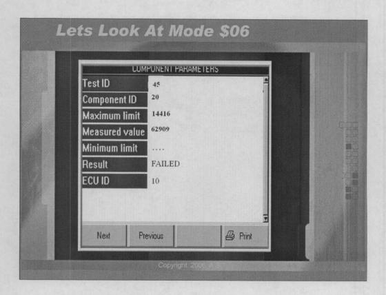
Looking at the Mode \$06 information on our scan tool, we see that the PCM has flagged the Test ID 45 as failed. TID 45 and CID 20 is the computer's test for a stuck open EGR valve. The test expects to see a voltage of less than .6 volts from the last reading it seen with the key on and engine off. If the voltage is higher, than it can safely assume there is a stuck open EGR valve present causing the voltage difference.
