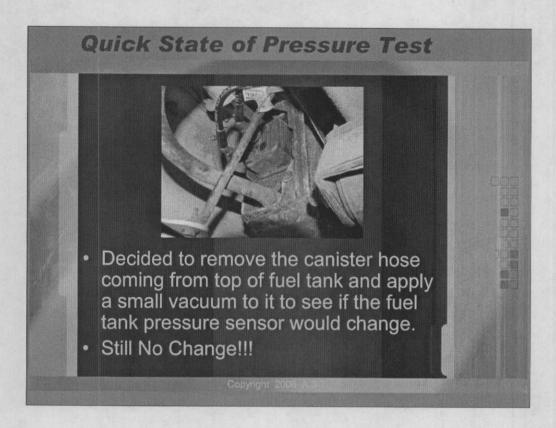
The quickest way to start gathering the information I was looking for was to raise the vehicle and remove the line that comes from the top of the fuel tank to the canister. I still had a scan tool displaying the pressure sensor reading and I tried to supply a small amount of vacuum to the line to see if I could get the reading on the scan tool to change. I still had no change from the fuel tank pressure sensor!
