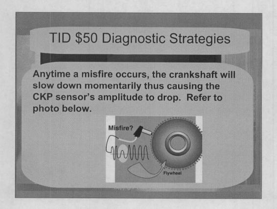
The PCM will monitor crankshaft speed by sampling the waveform emitted by the Crankshaft position sensor. Anytime a misfire occurs the crankshaft position sensor will produce a smaller amplitude signal. Since several things can cause the crankshaft to slow at times, the PCM will also generally look to the O2 sensor when it suspects a misfire is present. Remember, if a misfire did indeed occur, the exhaust will have a high level of oxygen since it did not get burned through the act of combustion.
