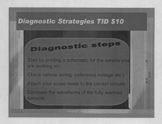
We want to begin our diagnostics by printing a wiring diagram for the vehicle we are working on. We see that the color of the wires that we wish to back-probe to attach our scope leads to in this case both happen to be the black wires coming directly off the sensors themselves.
