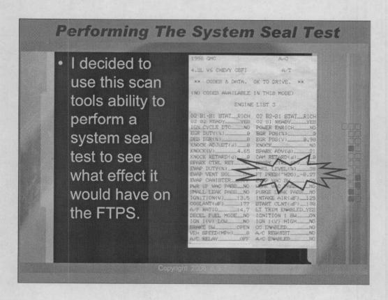
I figured the best place to start was to perform a system seal test using my scan tool and also monitoring the fuel tank pressure sensor for any changes over time. When I performed the system seal test I noticed that the value of the fuel tank pressure sensor did not change no matter what I did. Example: shake vehicle etc...
