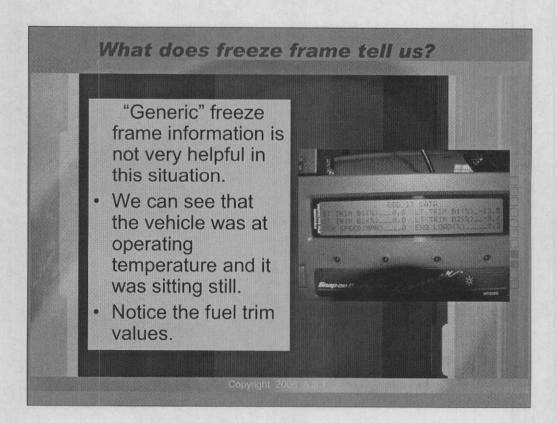
Freeze frame information is not of too much value to us in this case. The reason I chose to display this information is because the PCM will often look for changes in Idle Air Counts and Fuel Trim values to help determine if the system is operating correctly. This is just one of several tests that GM uses to test the integrity of the EVAP monitor.
