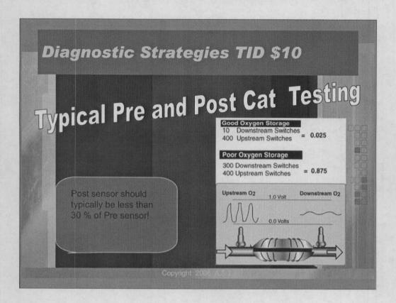
Typically, most OBD II vehicles will want to see that the amplitude (big slopes) and the frequency (half cycles) test of the catalyst sensor is 30% or less than the pre-cat sensor is displaying. If you have your scope leads attached properly to the pre and post sensors, you should be viewing a waveform similar to the one shown above.
