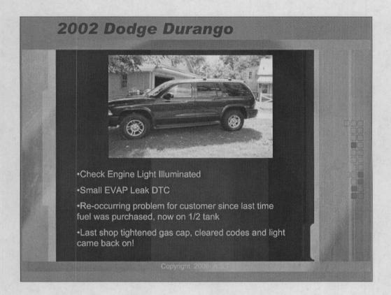
Our first vehicle is a 2002 Dodge Durango. This vehicle had already been to a service shop about one week earlier for an illuminated check engine light, which turned on shortly after the owner bought fuel. The shop checked for codes and determined that the gas cap was left loose so they tightened the cap and cleared the DTC.
