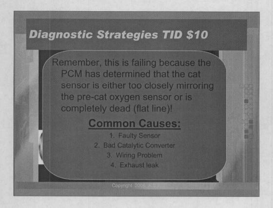
The most common causes for this condition are a faulty sensor, a bad converter, a wiring problem or an exhaust leak allowing pirate air into the exhaust stream thus influencing the sensor.
