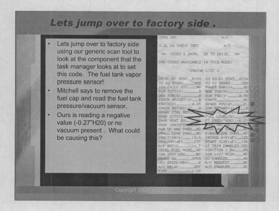
Lets jump over to factory side using our generic scan tool to look at the component that the PCM looks at to set this code. The fuel tank vapor pressure sensor!
