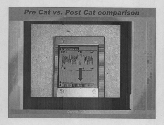
The above photo shows the actual pre and post catalytic sensor's waveforms. Remember that you can also use most scan tools to graph these signals as well. This is often a little easier to do since you only have to hook up to the ALDL.
