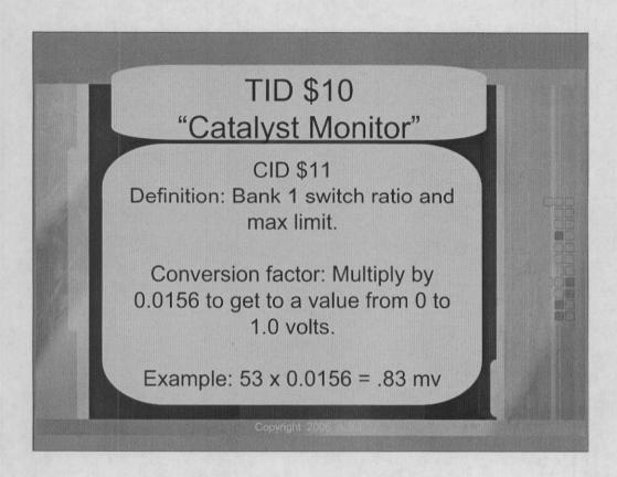
The above slide refers to the conversion factor that we must use with Ford vehicles that are not C.A.N. compliant. In order for us to get a voltage value from our Mode \$06 screen we must take the measured value of 3 and multiply that by 0.0156, which gives us a voltage value of 0.0468 millivolts. Remember, C.A.N. vehicles will have no conversion factor.
