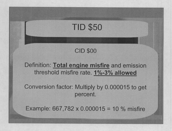
Test ID 50 is Ford's total engine misfire test found within Mode \$06. This test is usually the first to fail when a misfire is present. Eventually, we would fail a specific cylinder misfire test and thus begin to set diagnostic trouble codes. Ford has a testing procedure which allows approx. 3% total misfire to accommodate things such as road terrain etc.
