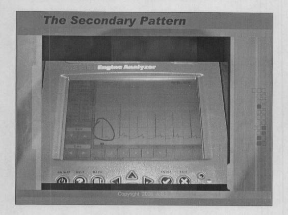
Once I had the ignition scope attached I initially saw nothing wrong with the waveform. I needed to drive the vehicle under several types of load conditions before I could get the miss to occur. Once the miss was present, it would come and go sporadically even at idle.
