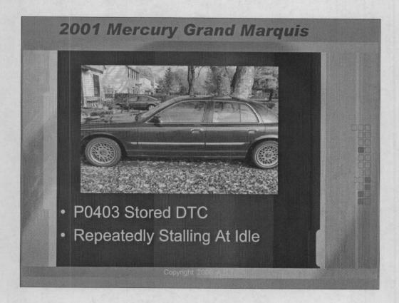
This next vehicle was an 01" Mercury that would not idle. We had a P0403 trouble code stored in the PCM's memory. This code represents a malfunction in the EGR's solenoid circuit. This code sets when the system is not in the correct state when the PCM is trying to run the EGR test. This can be caused by many things but with the complaint at hand, we would probably suspect a hanging open EGR valve due to carbon build-up or other debris.
