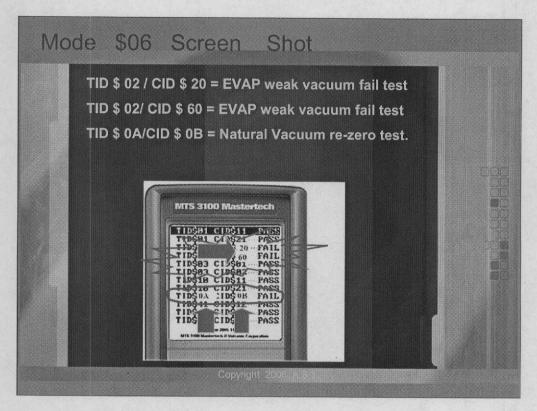
The Mode \$06 information has proved to be a real asset! We have three different failures present, which pertain to the EVAP monitor.
