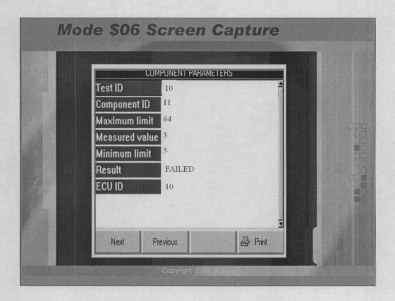
We then decided to view the Mode \$06 information and we see that the TID \$ 10 and CID \$ 11 has failed. Upon looking in our Mode \$06 diagnostics manual we also see that once this code sets, the PCM will stop running the EVAP test so we will have to be sure that once the vehicle is completed, not only does the catalyst monitor pass, but the EVAP monitor passes as well.
