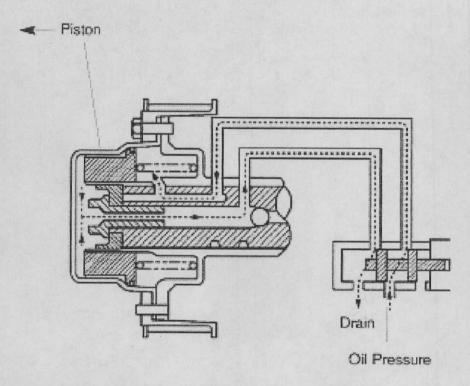
As the piston in the variable cam timing unit assembly is hydraulically pushed towards the front of the engine, the exhaust cam is in its advanced position.
