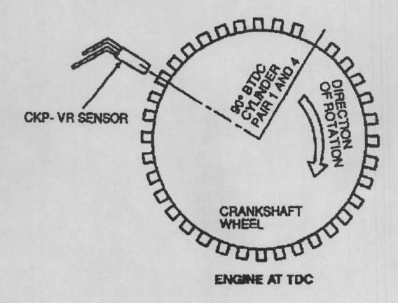
The crank synch pulse on the 36-1 tooth reluctor occurs  $90^{\circ}$  BTDC on the compression stroke of cylinder #1 in a 4-cylinder engine.
