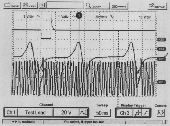
Channel 1 is on the "36 - 1" tooth crank sensor.
