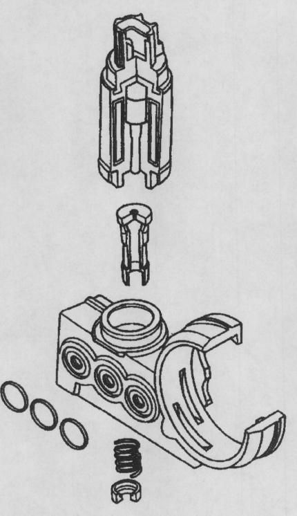
This is an exploded view of the VCT solenoid and oil feed flange assembly.
