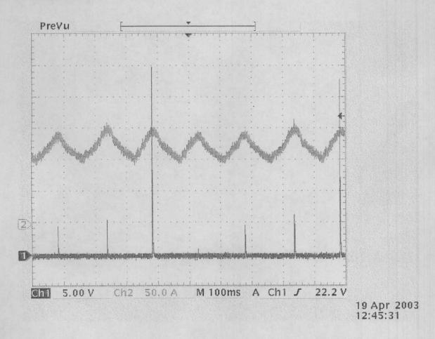
Channel 1 is connected to a synch probe clamped around the #1 plug wire, and Channel 2 is connected to a high amp current probe clamped around the battery cable. Fuel is disabled and the engine is cranking.
