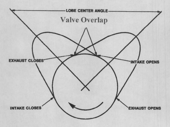
Valve overlap is defined as the amount of time that both the exhaust valve and the intake valve are open as the piston transitions from the exhaust stroke to the intake stroke.
