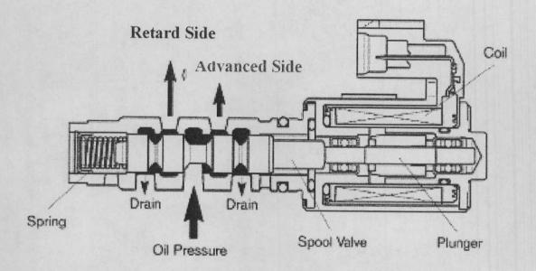
Engine oil pressure is supplied to the VCT solenoid. Depending on the PCM command, the VCT solenoid will direct oil to either the advanced side or the retarded side of the variable cam timing unit assembly (axially sliding piston).
