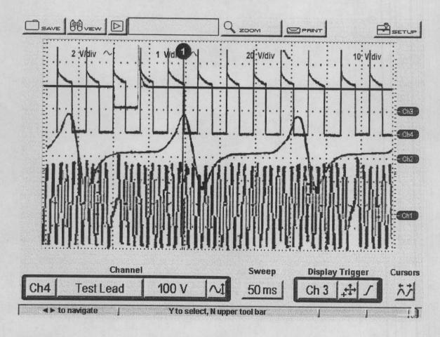
Channel 1 is on the "36 - 1" tooth crank sensor.
