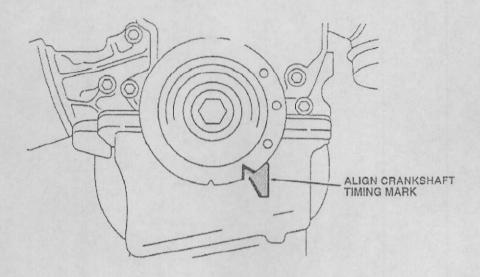
The first step in checking cam timing is to find TDC on compression for cylinder #1. There are marks on the harmonic balancer and aluminum bedplate.
