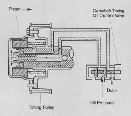
As the piston in the variable cam timing unit assembly is hydraulically pushed towards the rear of the engine, the exhaust cam is retarding its position from the timing belt sprocket.
