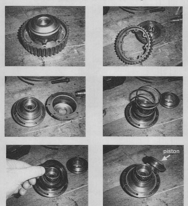
The helically splined piston connects the camshaft to the camshaft sprocket.
