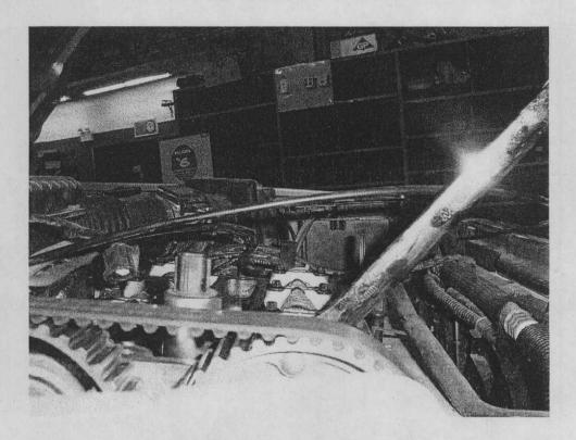
With the timing belt properly installed and the cam sprockets torqued, the exhaust cam can be rotated about 30°. This is normal.
