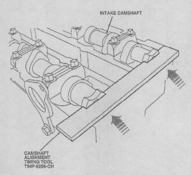
Once the crank is properly located, cam timing can be checked. An alignment tool should slide into the offset notches on the back side of both cams. A bar stock that is  $\frac{1}{4}$  inch thick by  $9-9\frac{1}{2}$  inches long by  $\frac{3}{4}-1$  inch wide will do the job.
