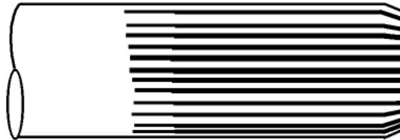
SPLINES WORN THIN WHERE AXLE ENGAGES GEAR
