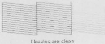
Nozzles are clean
