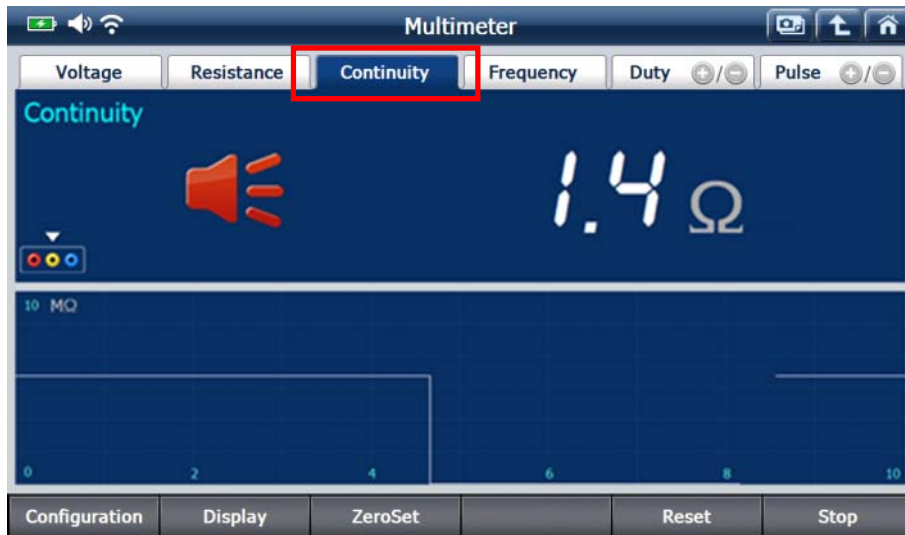
[ Continuity Test – Normal / Buzzer Sounds ]
