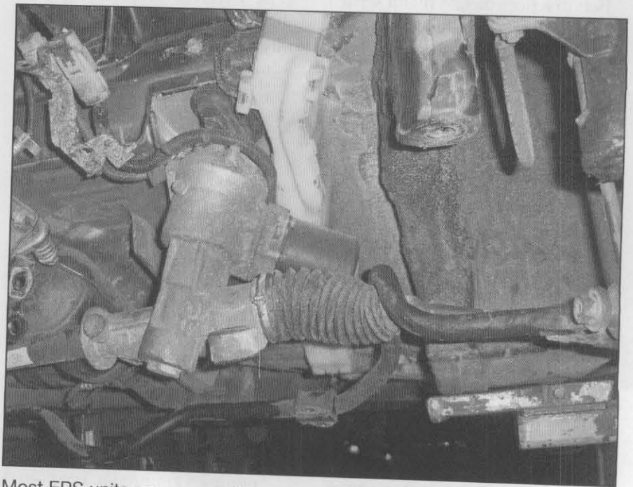
Most EPS units are operated by a 12-volt brush-type motor while some other vehicles will use a 42-volt version of EPS that receives its voltage from the HV converter.
