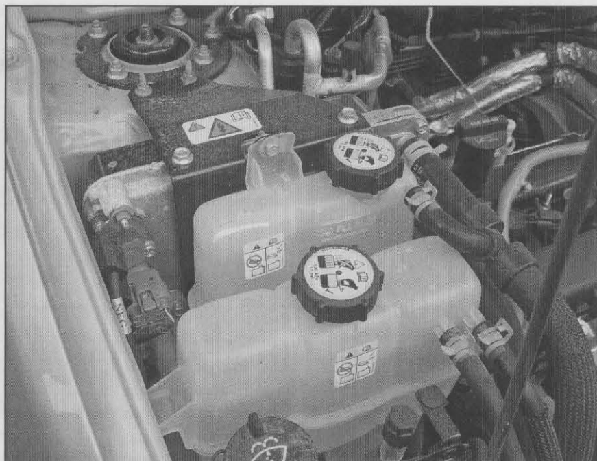
Coolant reservoirs are often located close together. On some models, other fluid reservoirs are also co-located with the coolant reservoirs.
