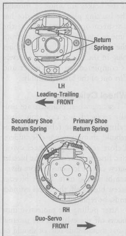
Brake shoe return spring design differences of leading-trailing and Duo-Servo drum brakes.
