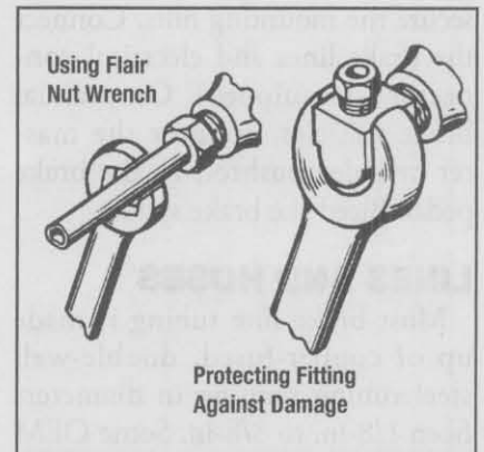
Using a flare nut wrench on a brake line fitting. (Courtesy: Bendix Corp.)
