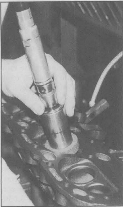
Grinding a valve seat with a wet stone.
