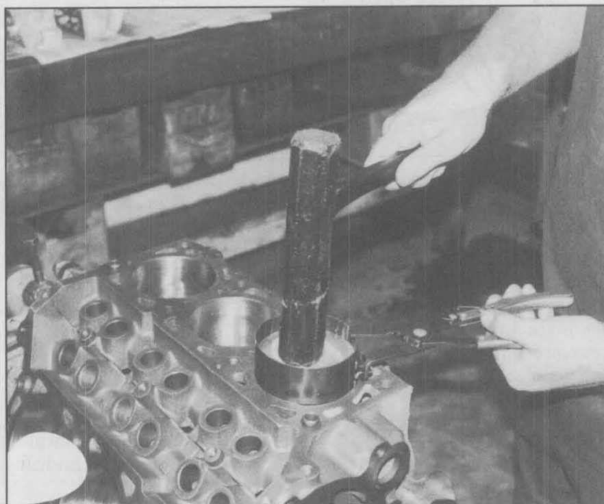
Using a ring compressor to install a piston into the cylinder block.
