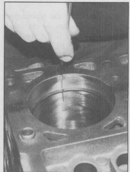
Measuring piston ring end gap.
