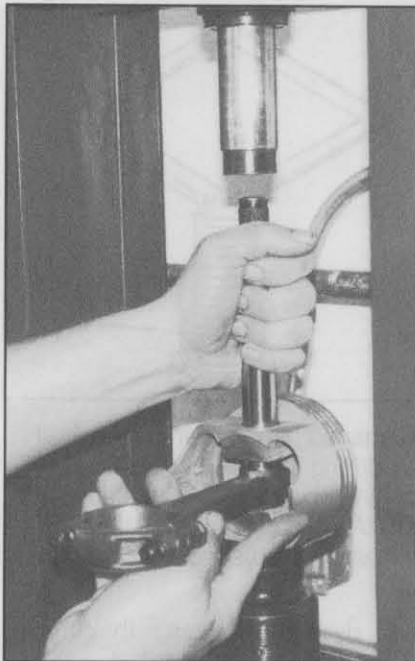
Pressing the piston pin into the connecting rod small end bore. A special fixture must be used to properly support the piston and locate the pin in the rod and piston pin bore.
